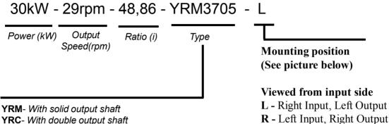
YRC- With double output shaft YRD- With hollow output shaft YRE- With extruder housing
