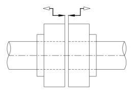
12-By fitting couplings be sure that there is no exantricity between the two shafts.
