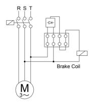
Delayed Running Brake 4 (24 V)
