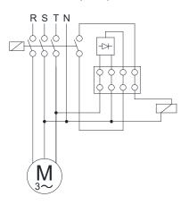
Delayed Running Brake ( 24 V)
