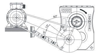
If direction of output shaft rotation is ccw;
