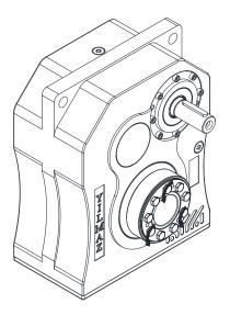
**7.7.2**- Use a solvent available in your market to clean all the dirt an oil from the shaft and shrink disk hollow. The surfaces must be free from oil or any dirt. The solvent must be removed from the surfaces as well.
