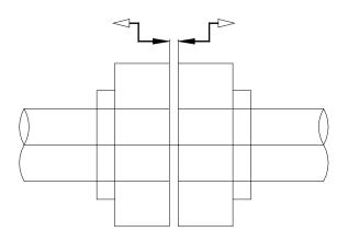
7.12.2-By fitting couplings be sure that there is no eccentric between the two shafts.
