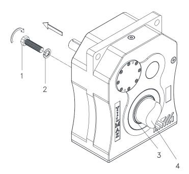
**7.3.2** -Use the disassemble set from YILMAZ and fasten the bold as shown bellow to take out the output shaft. For disassemble sets look the following pages.
