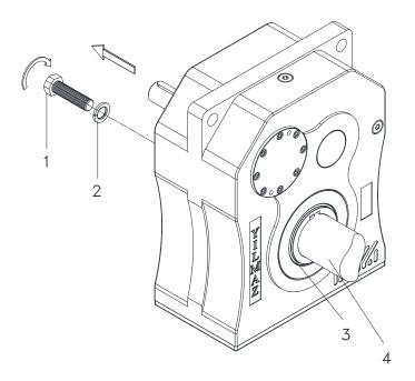
**7.4.2** -Use the disassembly set from YILMAZ and fasten the bold as shown bellow to take out the output shaft. For disassembly sets look the following pages.
