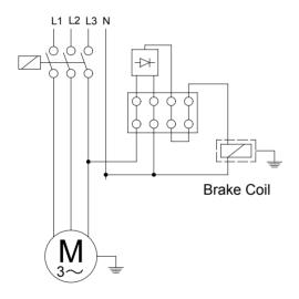
Delayed Running Brake (24 V)
