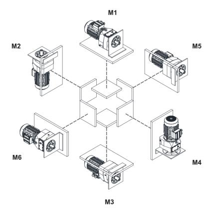
Indicated mounting positions are determined as reference directional position of the gearbox. Mounting surfaces are not binding.
