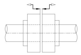
**7.3.2**- By fitting couplings be sure that there is no eccentricity between the two shafts.
